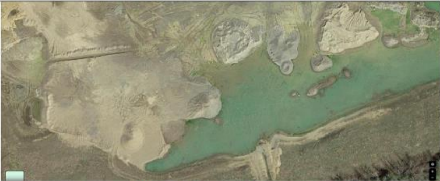
This view of the Southern Portion of The Pit shows the extent to which dredging was done to siphon off water from over excavated areas to below the water table.
